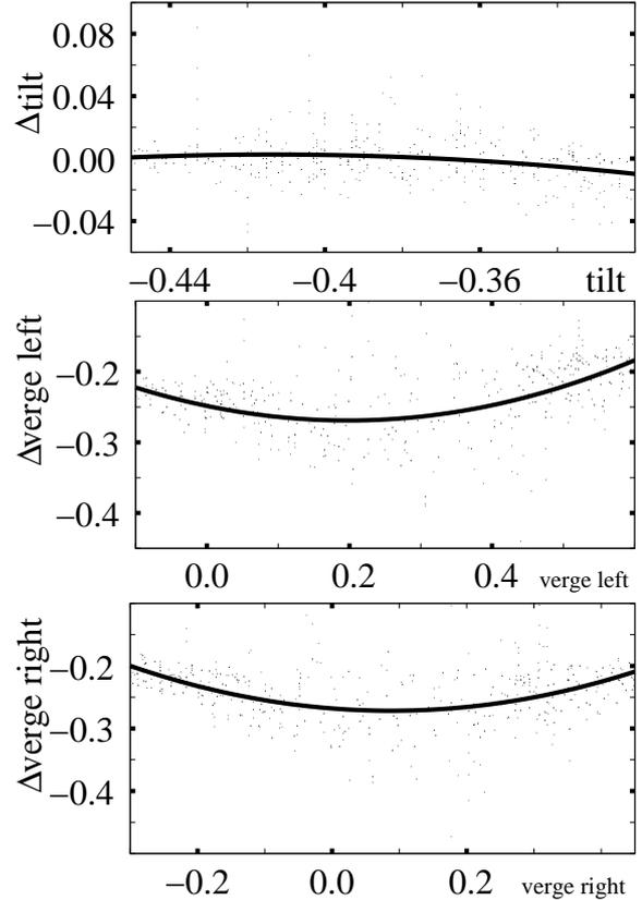
**Fig. 14** Empirical data representing the offset needed to shift the points in visual space in order to compensate the change from the centered to the shifted arm-vision configuration. The three diagrams show the offsets of a component over its absolute value for tilt (top), verge left (middle) and verge right (bottom). In addition the trend lines for the quadratic approximation is shown.
