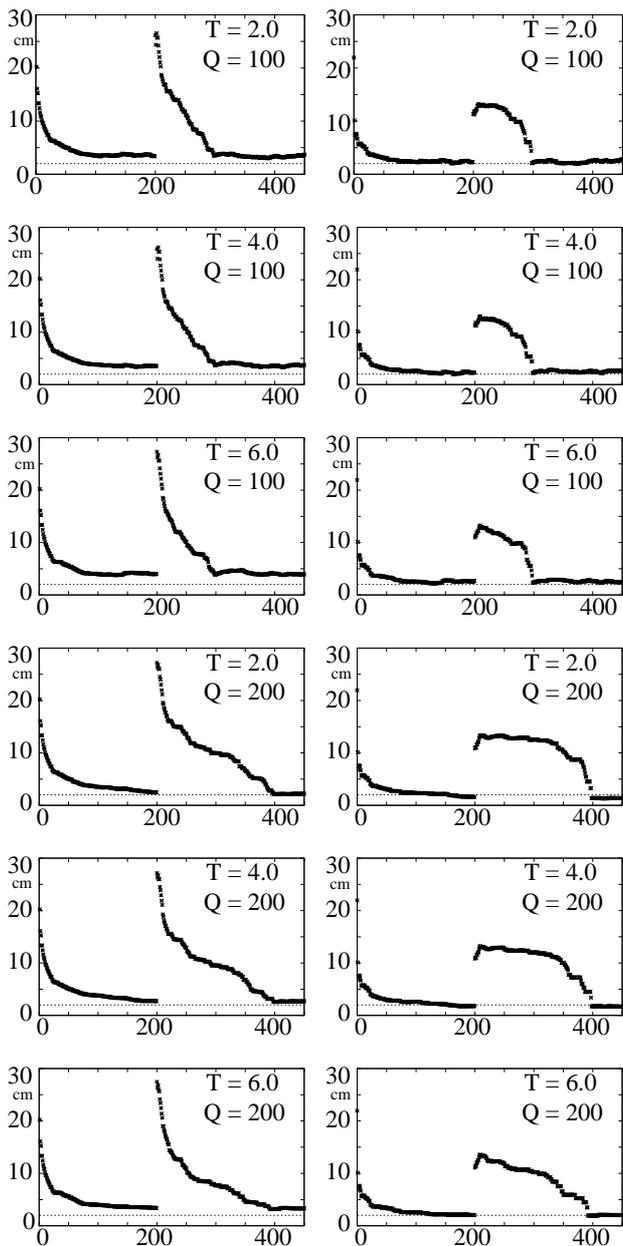
**Fig. 11** Average error (left) and standard deviation (right) of the table location ( $cm$ ) and its evolution over 450 cycles of the re-learning protocol for different  $Q$  and  $T$  values. The arm-vision configuration was altered after 200 cycles. These values result from an additional test sets (100 samples each). The base line in the diagrams on the left indicates the error level of  $2.0\text{ cm}$ .
