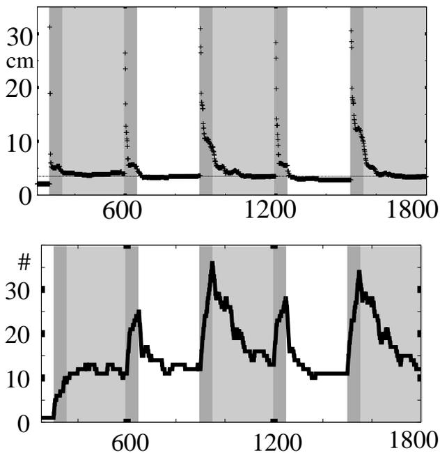
**Fig. 13** Evolution of average error (top) and number of links (bottom) resulting from architecture  $A_{\mathcal{S}}$  testing realignment over 1800 learning cycles for  $T = 8.0$  and  $Q = 50$  in the  $CP$  and  $SP$ . The base line in the top diagram indicates the value  $3.5$  cm. White regions represent the  $CP$ , light grey the  $SP$ .
